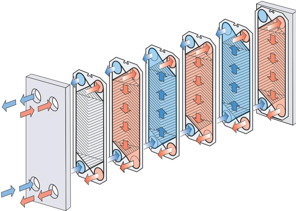
**Figure 2. Example of a single-pass set up.**
