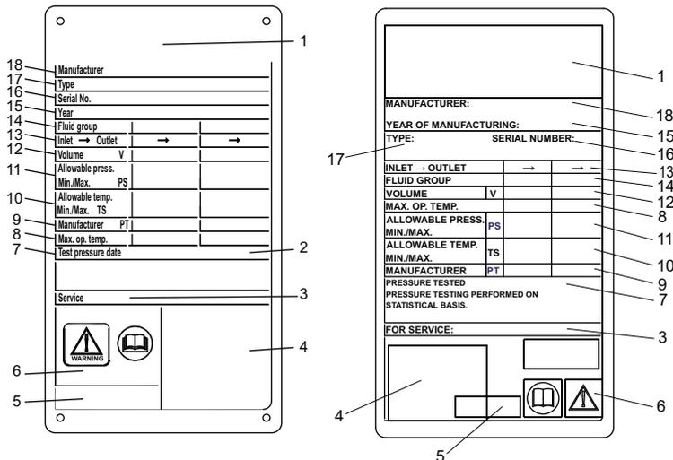
Figure 1. Example of CE metallic name plate to the left and CE sticker label name plate to the right
