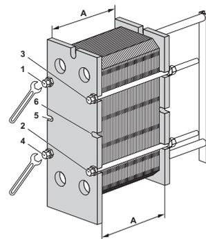
When a pneumatic tightening device is used, see table below for maximum torque. Measure dimension **A** during tightening.
