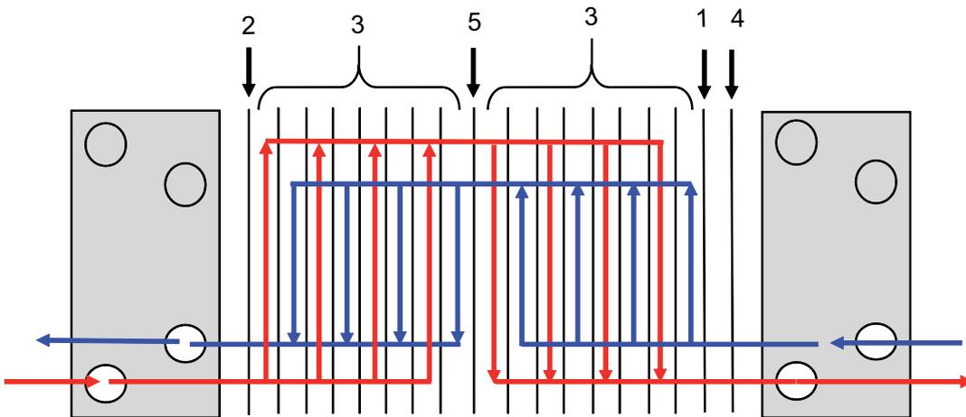
Figure 3. Example of a multi-pass set up
