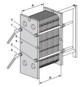
When a pneumatic tightening device is used, see table below for maximum torque. Measure dimension **A** during tightening.
