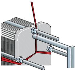
Figure 4. Lifting TS6
